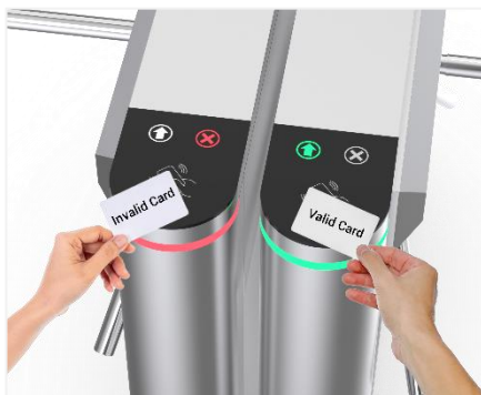
Green Arrow Indicator: swipe valid card Red X Indicator: swipe invalid card
